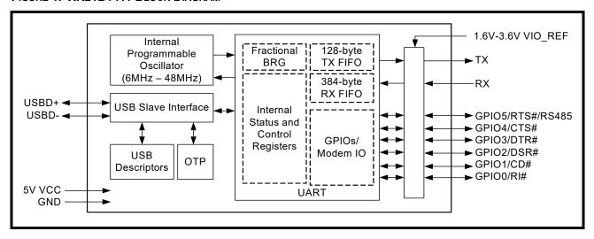
FIGURE 2. PIN OUT DIAGRAM
