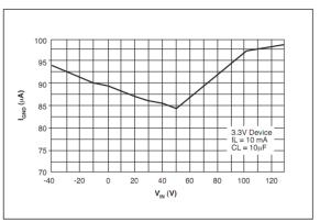
Fig. 7: Ground Current vs Input Voltage
