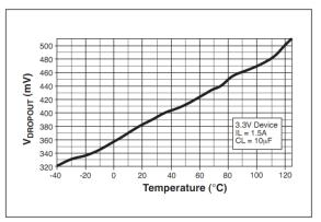
Fig. 17: Dropout Voltage vs Temperature  $$I_{\text{LOAD}}$=$1.5A$$
