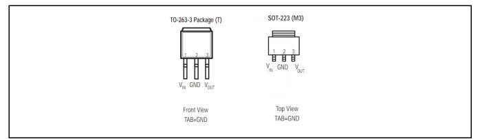
Fig. 3: SPX3940 Pin Assignment
