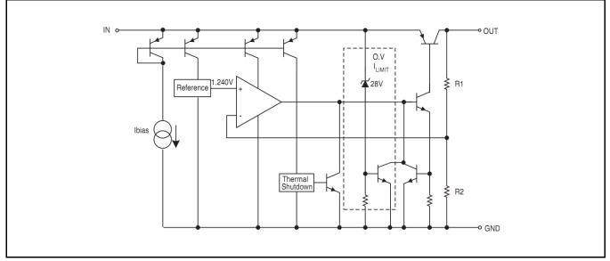
Fig. 2: SPX3940 Block Diagram
