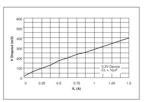
Fig. 9: Dropout Voltage vs Load Current
