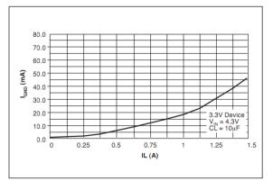
Fig. 6: Ground Current vs Load Current
