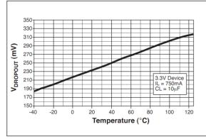
Fig. 16: Dropout Voltage vs Temperature  $I_{\text{LOAD}}{=}750\text{mA}$
