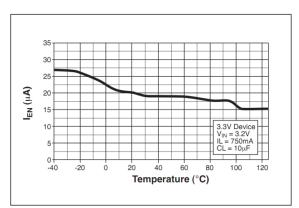
Fig. 18: Enable Current vs Temperature  $$V_{\text{EN}}$=$16V$
