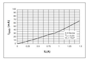
Fig. 8: Ground Current vs Load Current in Dropout
