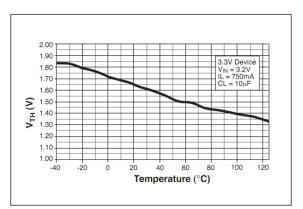
Fig. 19: Enable Threshold vs Temperature
