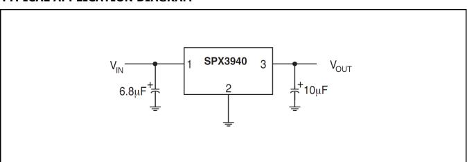
Fig. 1: SPX3940 Application Diagram – Fixed Output Linear Regulator
