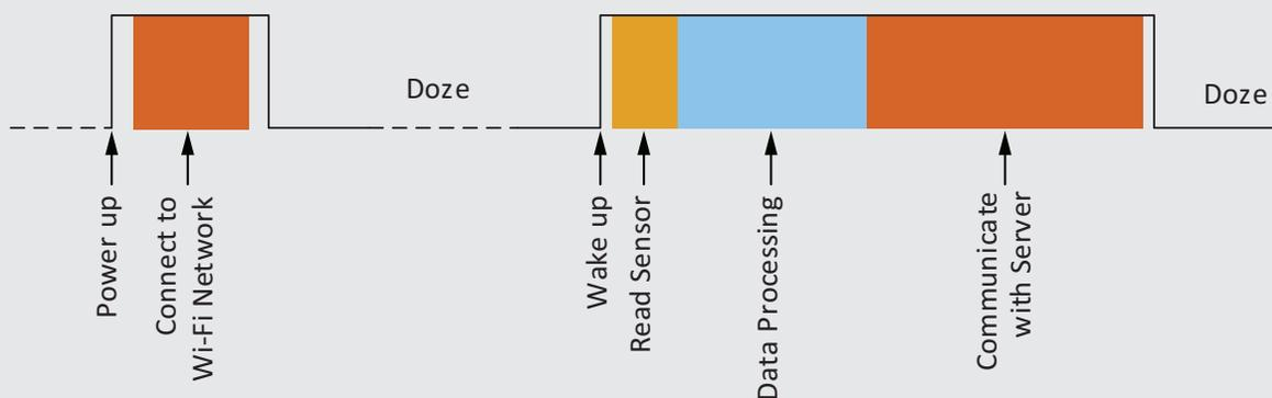
*Wi-Fi is the most convenient way for IoT devices to connect to the internet. The diagram shows that the bulk of time a device consumes power from the battery is when communicating with the server. The newer Wi-Fi standard reduces the time an IoT device spends awake for communication.*
