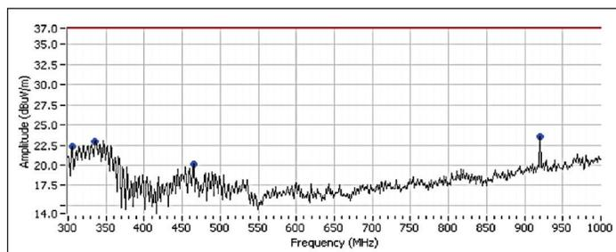
Figure 4. EMI Test Without Input/Output Filters
