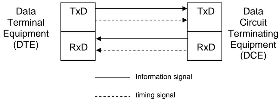
**Contra-Directional Timing:** A configuration in which a timing signal and associated binary signals (data or control) are transferred in opposite directions across the interface. This configuration would apply to Transmit Clock/Data only.
