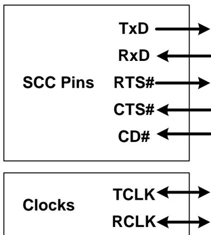
The signal names and directions reflect their function in a DTE configuration, but an SCC may be programmed to operate as either DTE or DCE.
