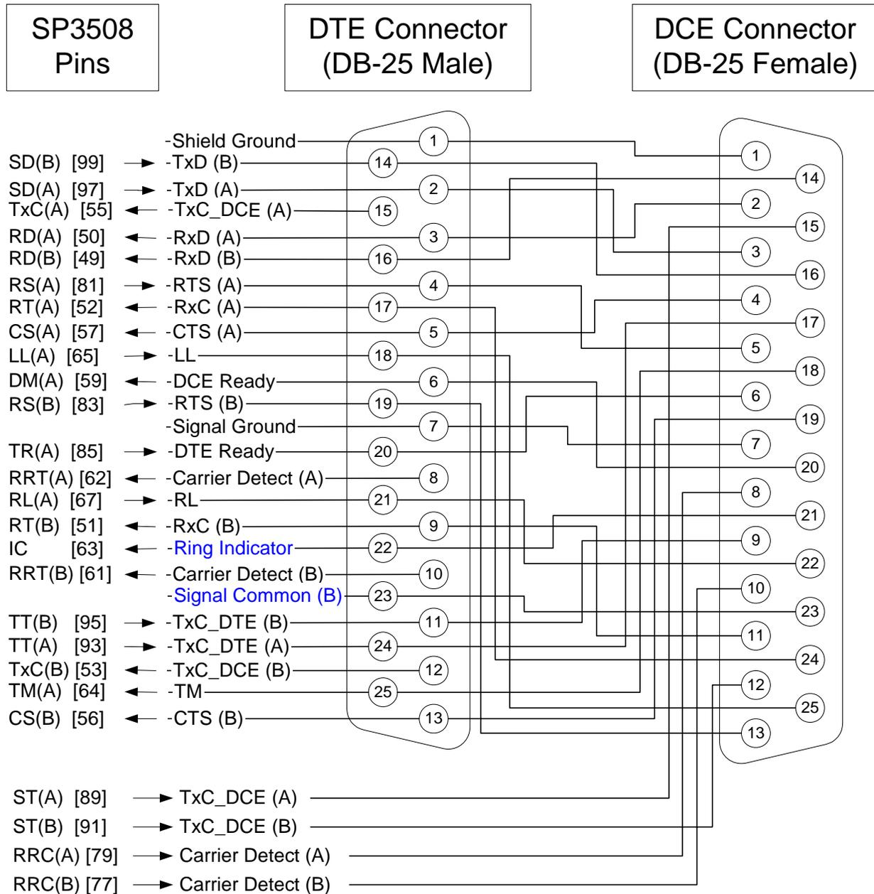
The figure above shows the standard pin connections between SP3508 and the DB-25 connector specified in ANSI/TIA/EIA-530-A (1991). A male connector is specified for the DTE and a female connector for the DCE.
