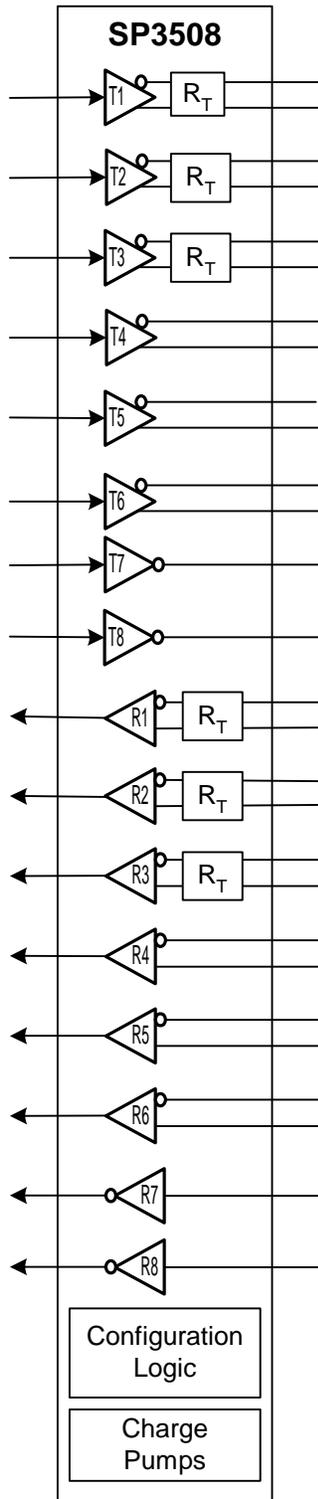
The SP3508, SP508 and SP509 are all highly integrated multiprotocol serial transceivers. Each have a total of 8 drivers and 8 receivers and can be configured to support a variety of standard serial port standards.
