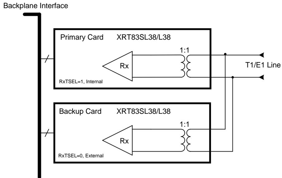
**Figure 2a. Simplified Block Diagram of the Receive Section for a 1:1 Redundancy Scheme Using Two Transformers**
