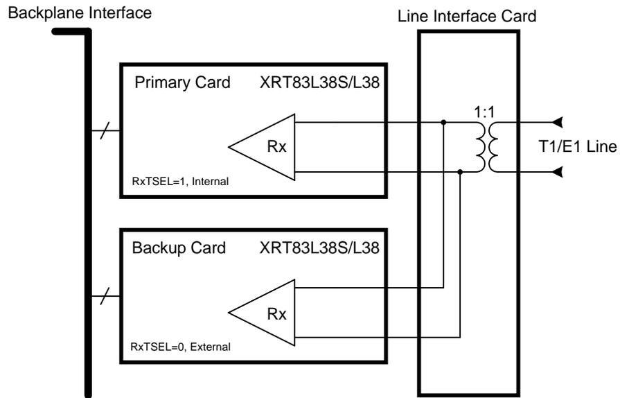
**Figure 2b. Simplified Block Diagram of the Receive Section for a 1:1 Redundancy Scheme Using One Common Transformer**
