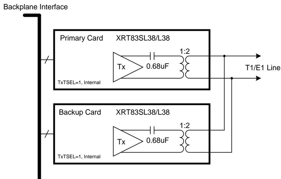
**Figure 1a. Simplified Block Diagram of the Transmit Section for a 1:1 Redundancy Scheme Using Two Transformers**
