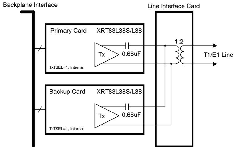
**Figure 3b. Simplified Block Diagram of the Transmit Section for a 1+1 Redundancy Scheme Using One Common Transformer**
