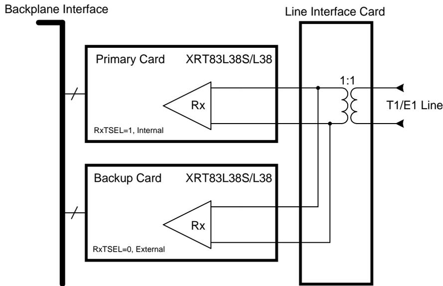
**Figure 4b. Simplified Block Diagram of the Receive Section for a 1+1 Redundancy Scheme Using One Common Transformer**
