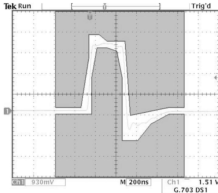
Figure 8 Pulse Template for T1 100ohm Impedance
