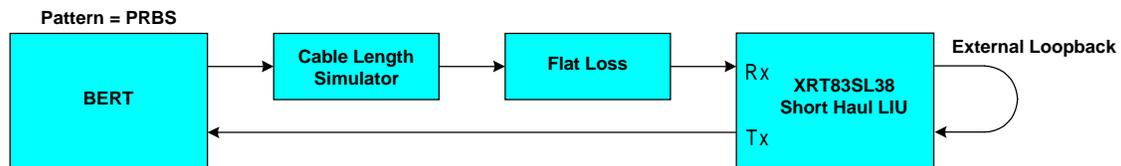
Figure 10 Simplified Lab Setup for Receive Sensitivity Measurements
