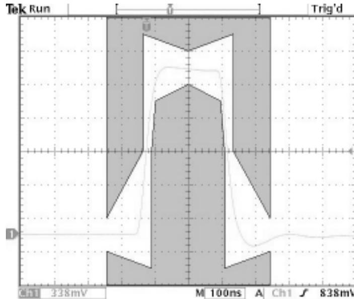
Figure 9 Pulse Template for E1 75ohm Impedance
