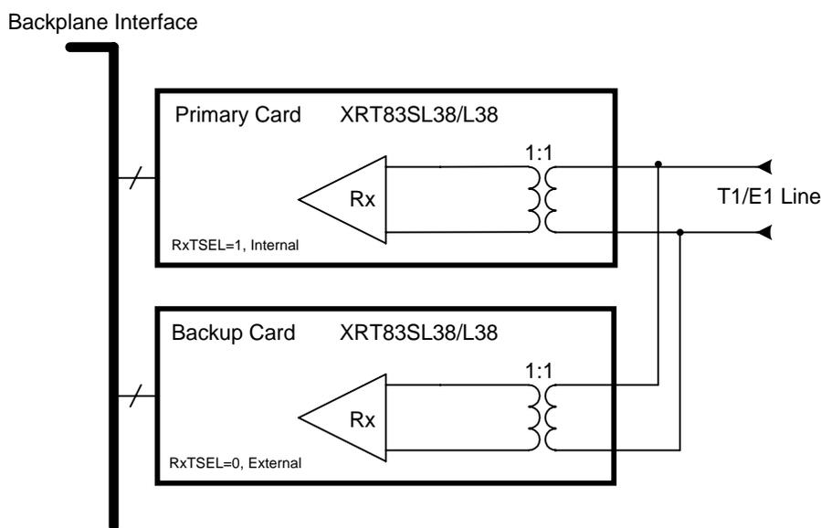
**Figure 4a. Simplified Block Diagram of the Receive Section for a 1+1 Redundancy Scheme Using Two Transformers**
