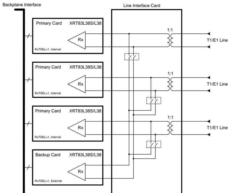
Figure 6. Simplified Block Diagram of the Receive Section for an N+1 Redundancy Scheme
