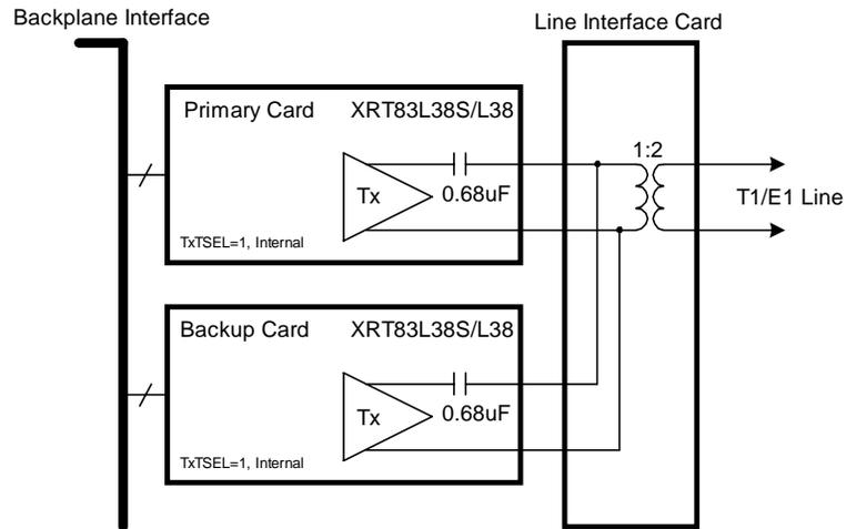
**Figure 1b. Simplified Block Diagram of the Transmit Section for a 1:1 Redundancy Scheme Using One Common Transformer**
