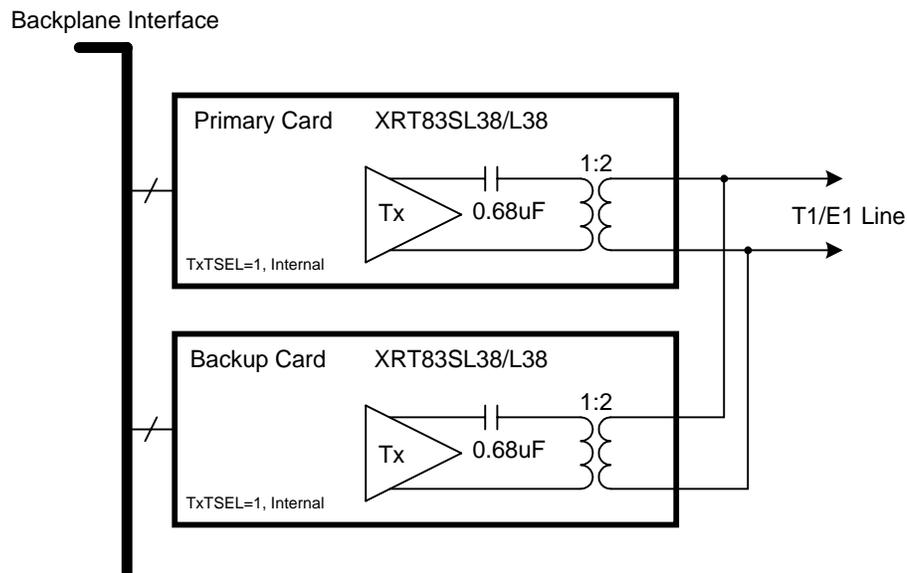
**Figure 3a. Simplified Block Diagram of the Transmit Section for a 1+1 Redundancy Scheme Using Two Transformers**
