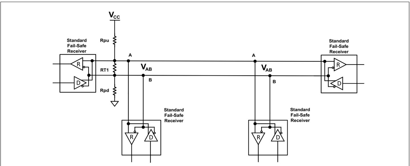
**Figure 4: Standard Fail-Safe Receiver with Termination Resistors Network**
