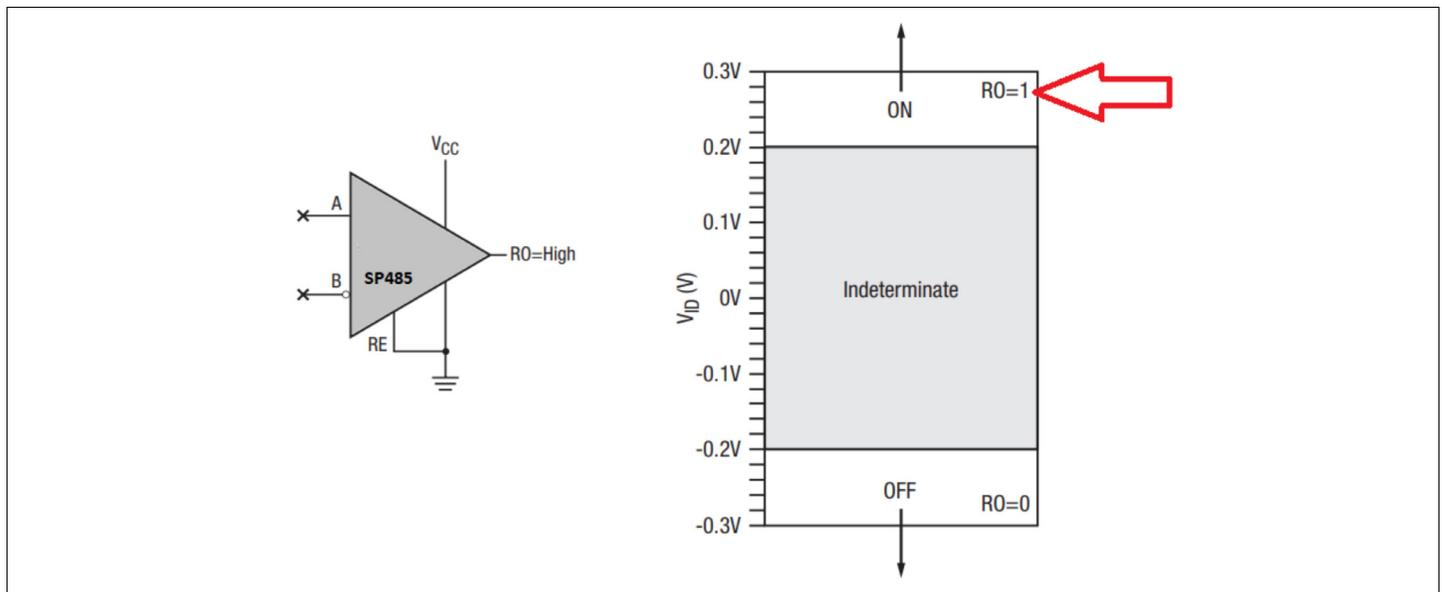
**Figure 1: Standard Fail-Safe Receiver with Open Inputs**
