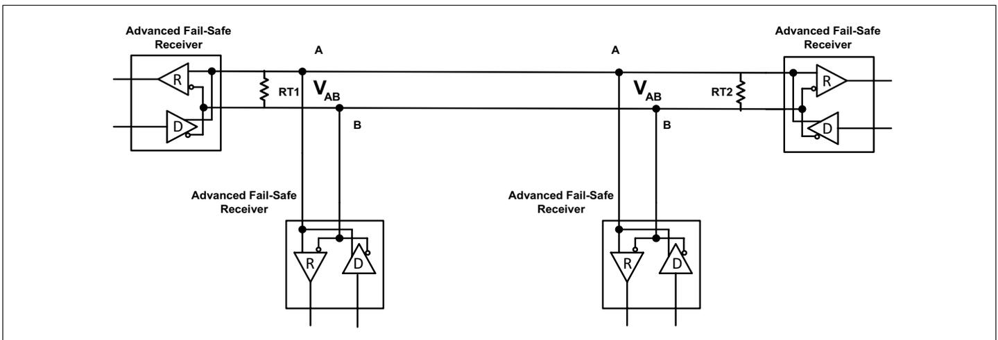
**Figure 7: Advanced Fail-Safe Receiver Typical System Connections**
