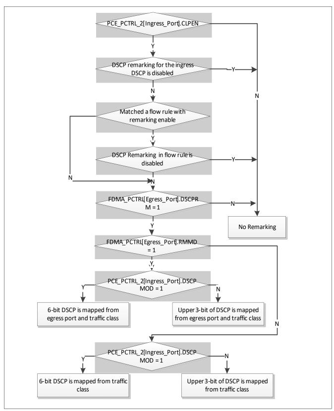
Figure 33 DSCP Remarking Flow Diagram
