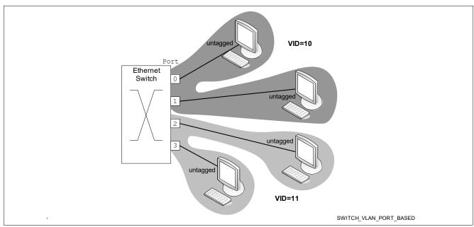
Figure 28 Port-based VLAN Example
