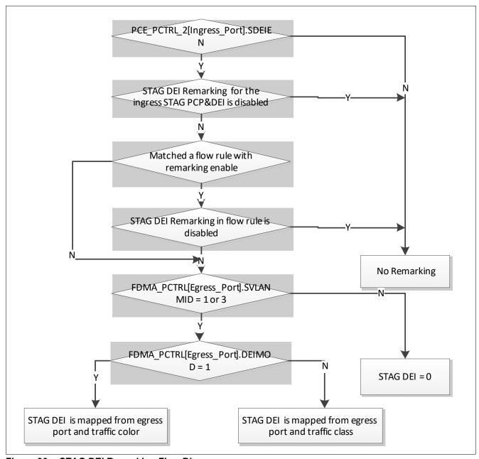
Figure 36 STAG DEI Remarking Flow Diagram
