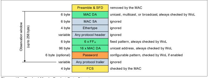
Figure 43 Typical Magic Packet Data Structure
