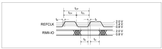
Figure 50 Transmit/Receive Timing Diagram of the RMII
