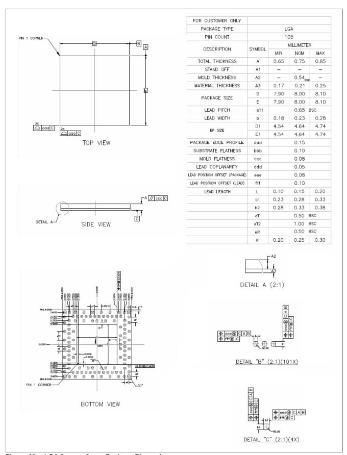
Figure 60 LGA 8 mm x 8 mm Package Dimensions
