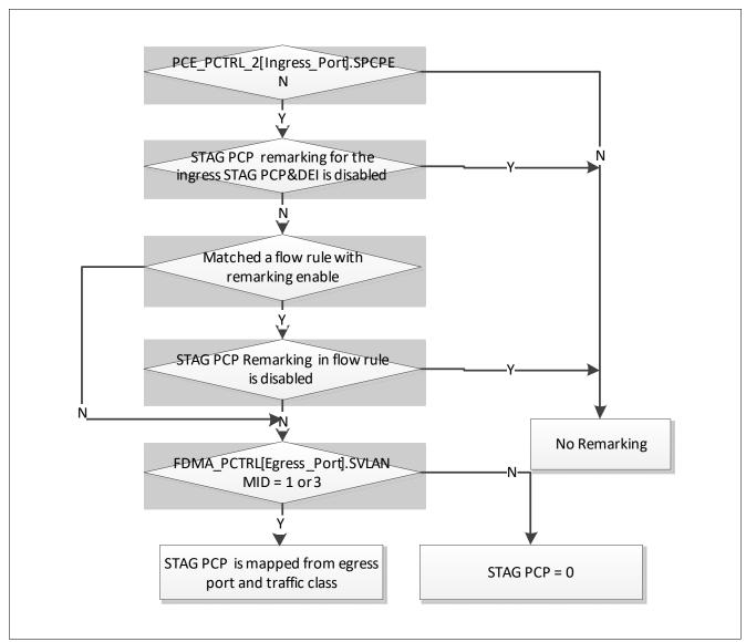
Figure 35 STAG PCP Remarking Flow Diagram
