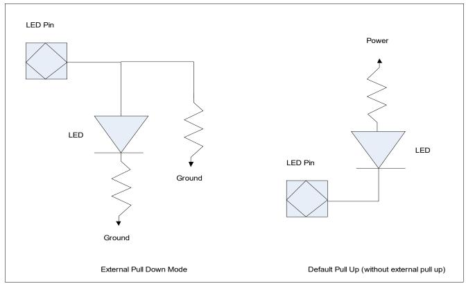
Figure 13 Pin Strapping on Single Color LED
