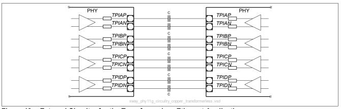
Figure 19 External Circuitry for the Transformerless Ethernet Application
