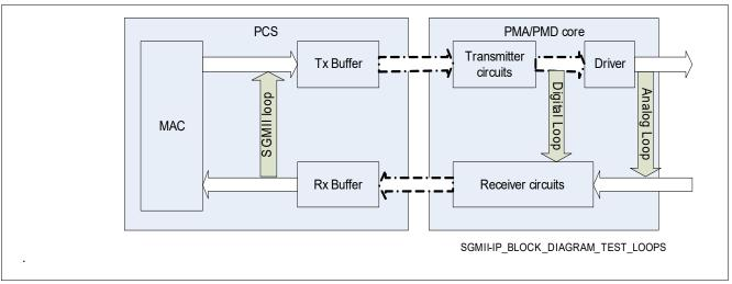
Figure 22 Test Loops in the GSW120
