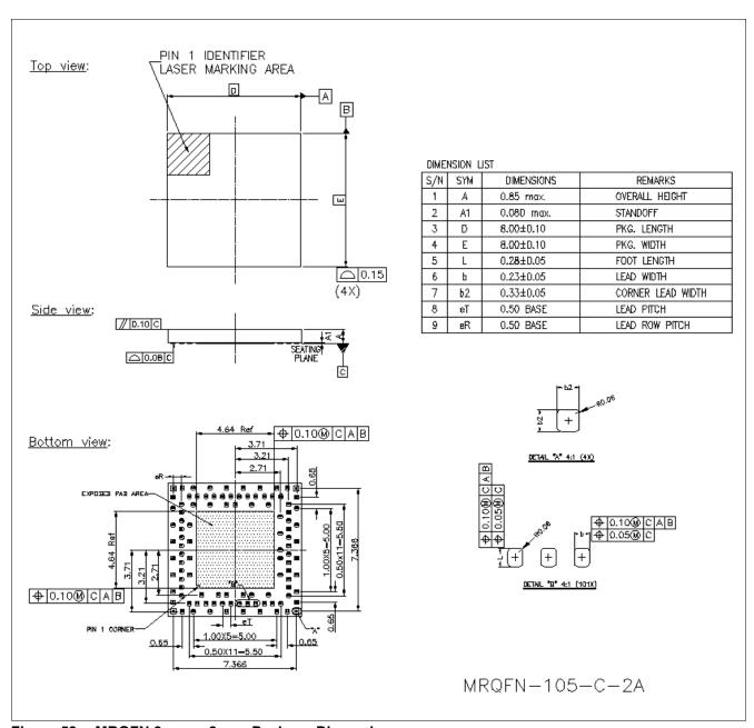
Figure 58 MRQFN 8 mm x 8 mm Package Dimensions
