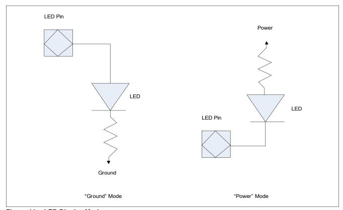
Figure 11 LED Display Mode
