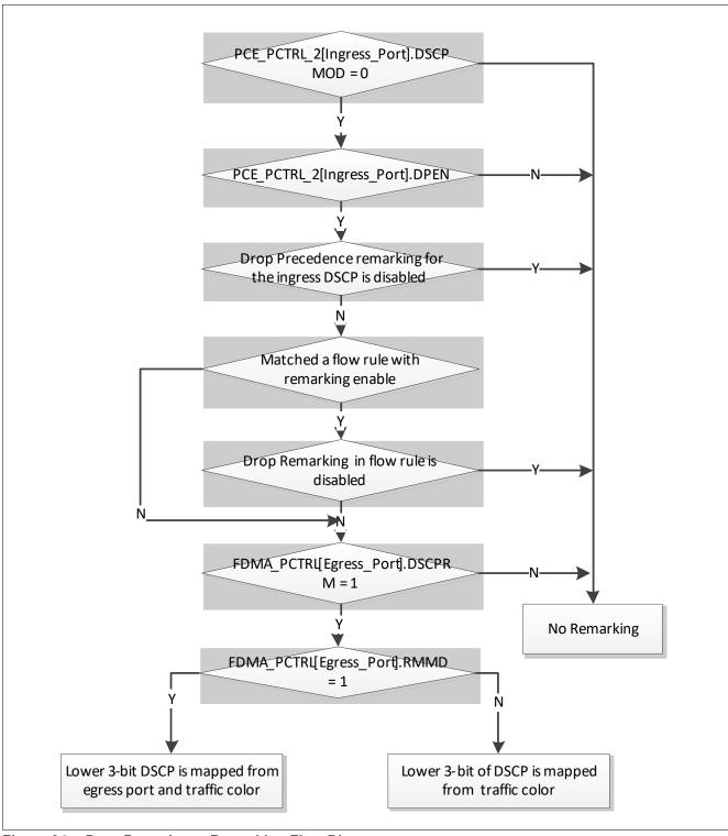
Figure 34 Drop Precedence Remarking Flow Diagram
