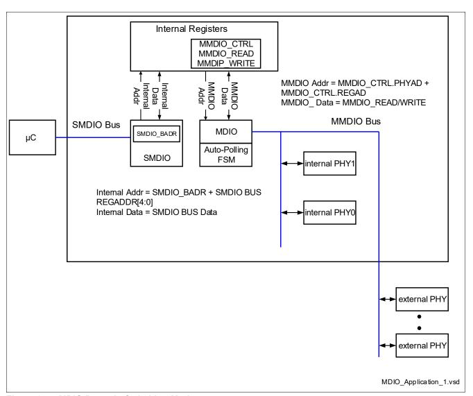
Figure 9 MDIO Proxy in Switching Mode
