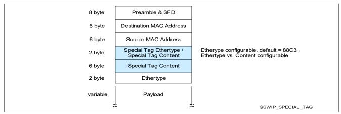
Figure 46 Special Tag Location in the Frame
