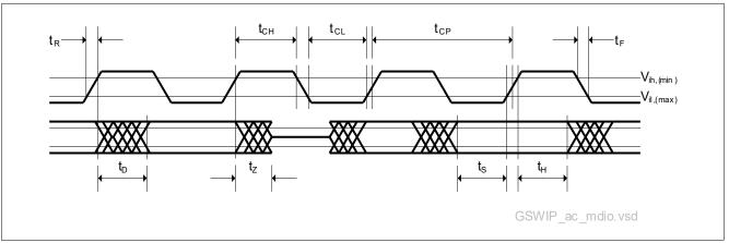
Figure 49 Timing Diagram for the SMDIO Interface
