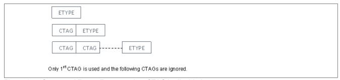
Figure 27 Supported Frame Formats when STAG is disabled
