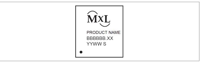
Figure 61 Example of Chip Marking
