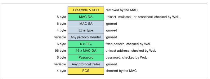
Figure 44 Magic Packet Data Structure - Password Protection
