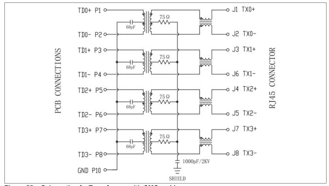
Figure 55 Schematic of a Transformer with CMC on Line
