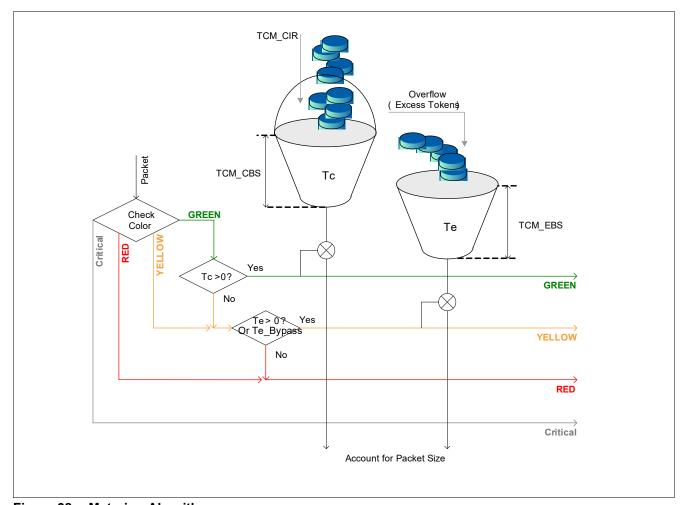
Figure 38 Metering Algorithm
