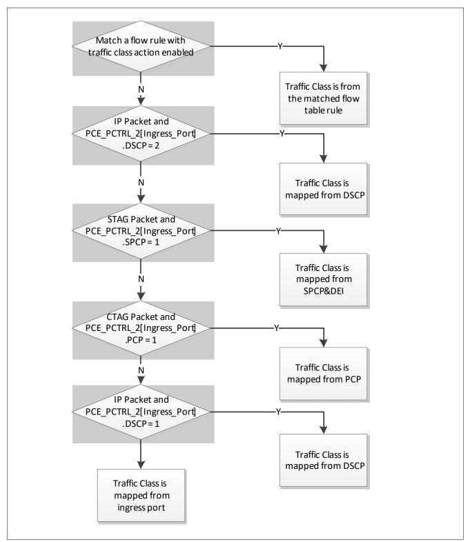
Figure 31 Traffic Class Assignment
