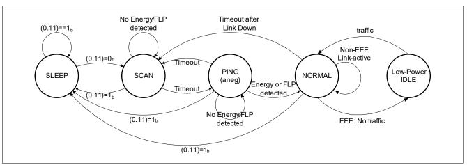
Figure 20 State Diagram for Power-Down Mode Management
