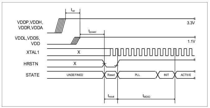
Figure 47 Timing Diagram for the GSW120 Reset Sequence
