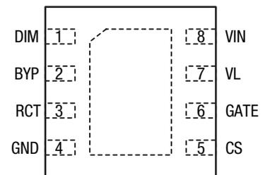
3mm x 3mm DFN-8L, Top View
