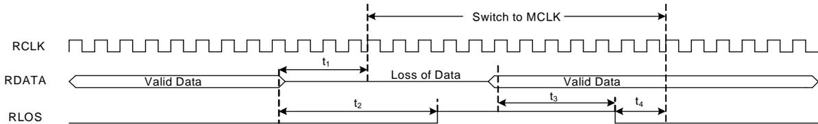
**Figure 1. PLL Recovered Clock Timing**
