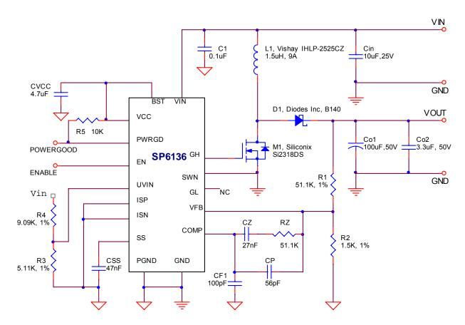
Figure 1- Boost converter based on SP6136, VIN=7 to 18V, VOUT=28V, IOUT=0 to 0.5A, converter operates at Discontinuous Current Mode under all line and load conditions
