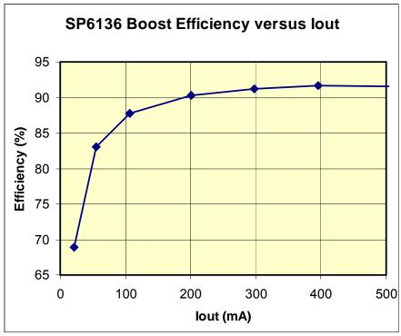
Figure 5- Efficiency at VIN=12V
