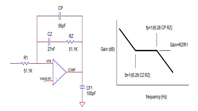
Figure 4- Error Amplifier (EA) and its transfer function for type II compensation, components shown are redrawn from figure 1, Error Amplifier is internal to SP6136 controller.
