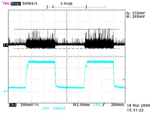
Figure 7- Step load response, I1=50mA, I2=500mA, f=1KHz, D=0.5, Ch1=Vout, Ch4=Iout
