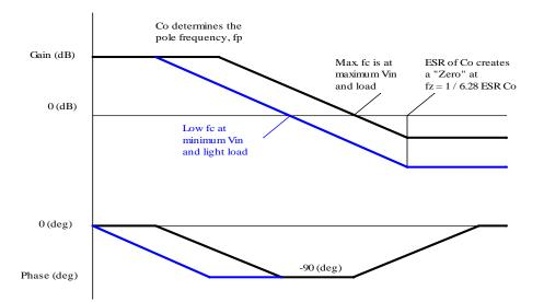
Figure 2- Control-to-Output transfer function of DCM boost converter, Gain/phase corresponding to low VIN and light load are shown in blue.
