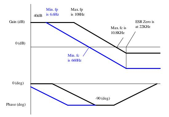
Figure 3- Design example Control-to-output transfer function, gain/phase corresponding to VIN=7V and Io=50mA are shown in blue.
