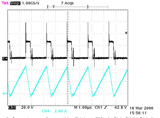
Figure 8- Converter waveforms at VIN=7V, IOUt=500mA, Ch1=SWN, Ch4=IL
