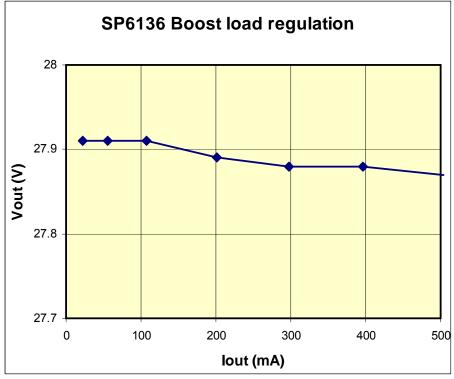
Figure 6- Load regulation at VIN=12V
