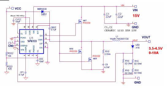
Note: ISP and ISN are shorted to ground. When using the SP6133 with output voltages above 3.3Volts the overcurrent feature of the part cannot be used and these pins should be shorted to ground.
