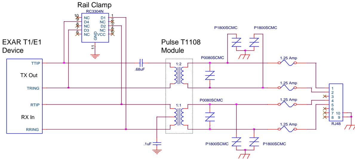
**Figure 3. Reference Schematic for GR-1089 Protection – Inter-Building Applications With Power Feed on Twisted Pair**
