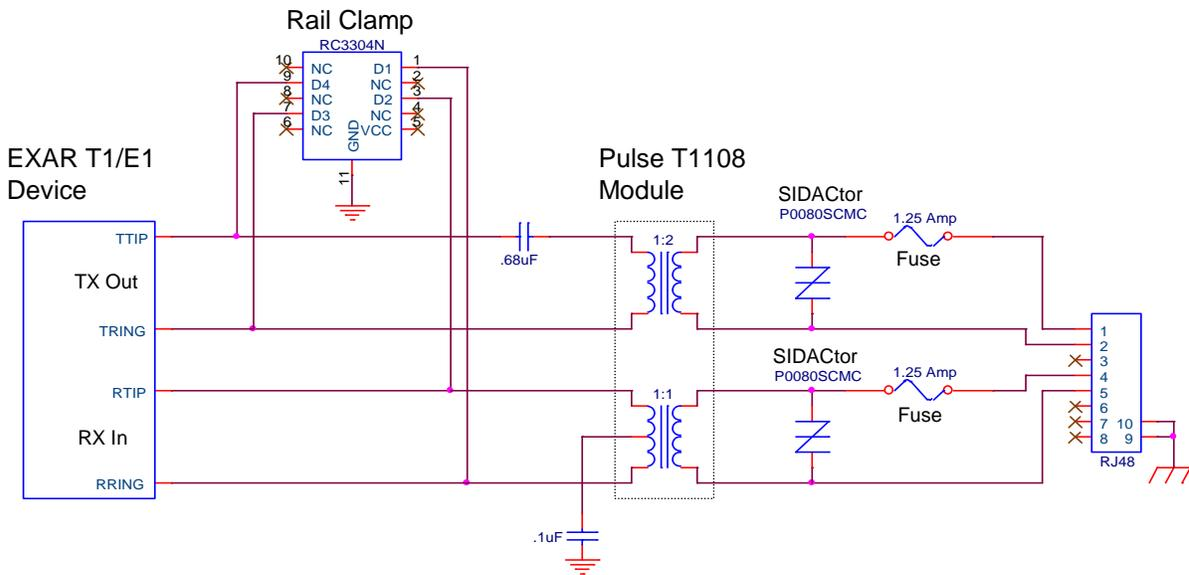
**Figure 2. Reference Schematic for GR-1089 Protection – Applications Without Power Feed on Twisted Pair**
