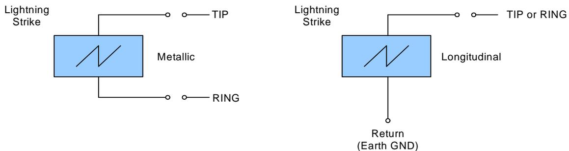
**Figure 1. Metallic and Longitudinal Modes**
