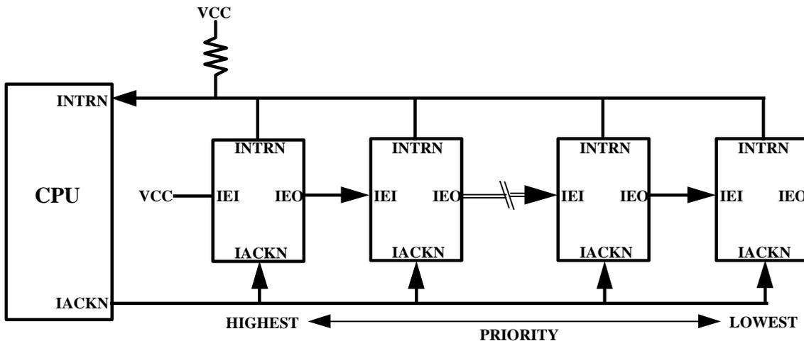
**Figure 1, An Illustration of XR-88C681 devices operating in a Daisy Chain, when commanded into the Z-Mode.**
