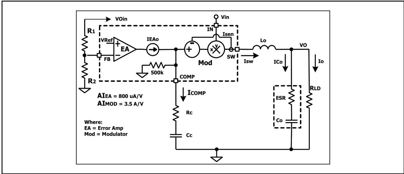
Fig. A1: Circuit Diagram
