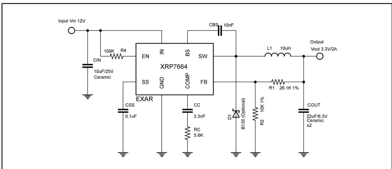
Figure 1: Datasheet Application Circuit
