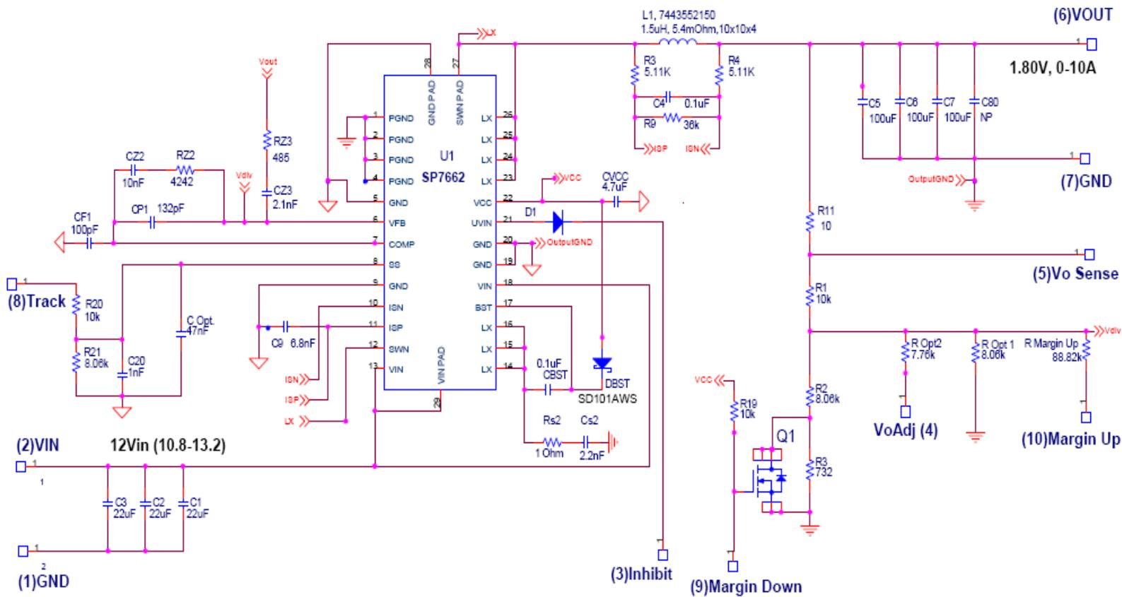
Figure 7 – Final Schematic
