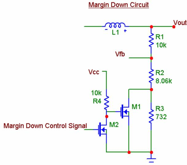
Figure 6 – Margin Down Circuit
