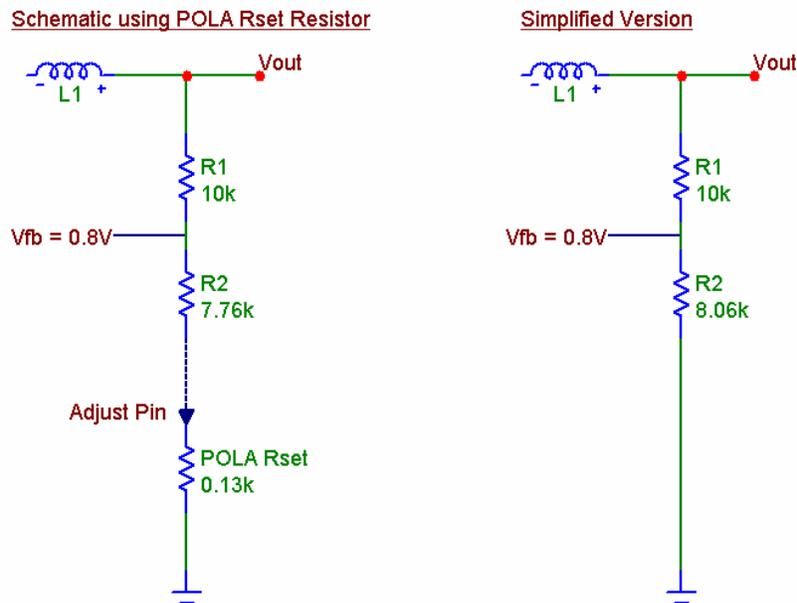
Figure 2 – Setting the Output Voltage
