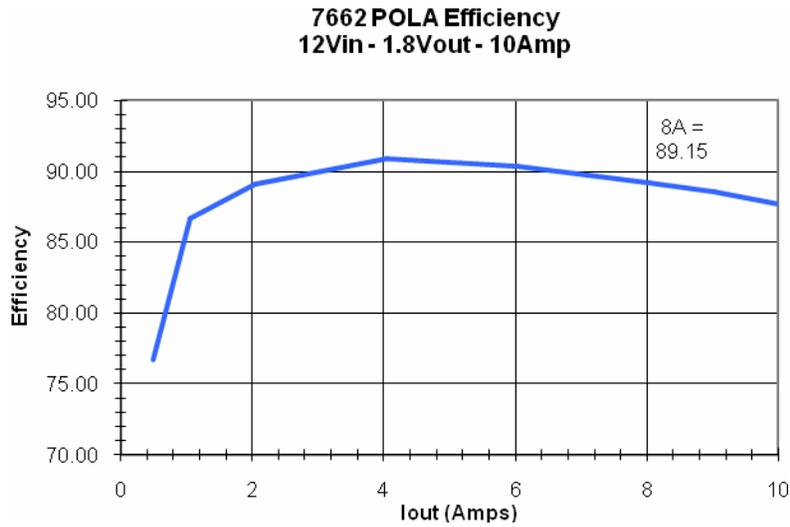
Figure 8 – Design Efficiency (POLA™ quoted efficiency at 8Amp = 87%)
