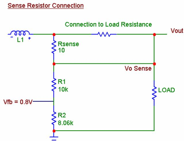
Figure 3 – Placement of Sense Resistor
