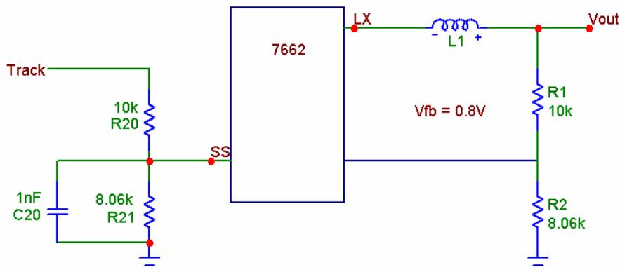
Figure 4 – Track Feature Connection diagram
