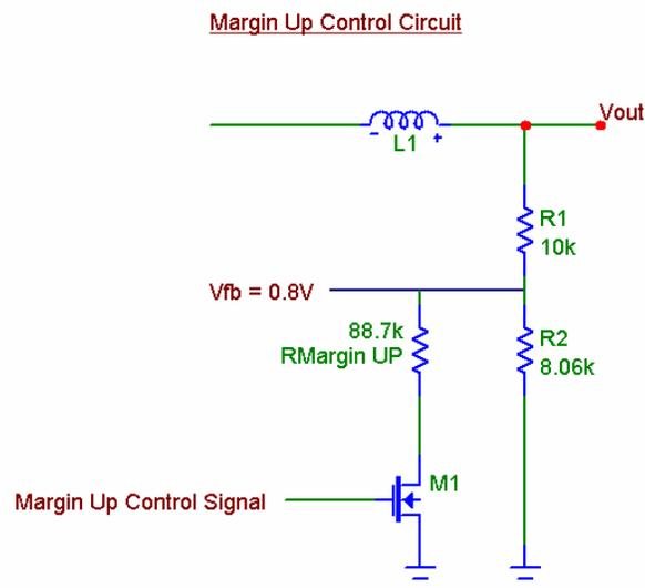
Figure 5 – Margin Up Resistor Connection
