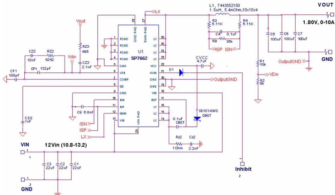
Figure 1 – Core DC-DC Converter Design
