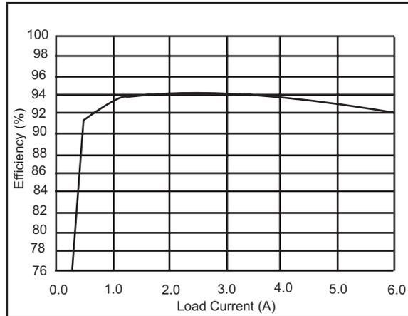
Figure 2. Efficiency versus Load Current for SP7652 at 5V<sub>IN</sub> and 3.3V<sub>OUT</sub>
