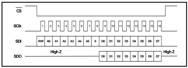
**Note:** If the R/W bit is set to "1", then this denotes a "READ" operation with the Microprocessor Serial Interface. Conversely, if the R/W bit is set to "0", then this denotes a "WRITE" operation.
