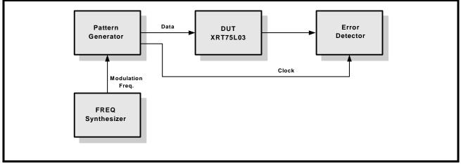
Input jitter tolerance requirements are specified in terms of compliance with jitter mask which is represented as a combination of points.Each point corresponds to a minimum amplitude of sinusoidal jitter at a given jitter frequency.
