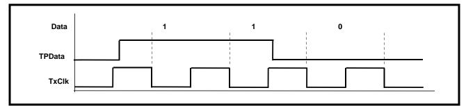
• In Dual-Rail mode, data is input via TPData\_n and TNData\_n pins. TPData\_n contains positive data and TNData\_n contains negative data. The SR/DR input pin = "Low" (in Hardware Mode) or bit 0 of channel register = "0" (in Host Mode) enables the Dual-Rail mode. Figure 13 illustrates the Dual-Rail data format.
