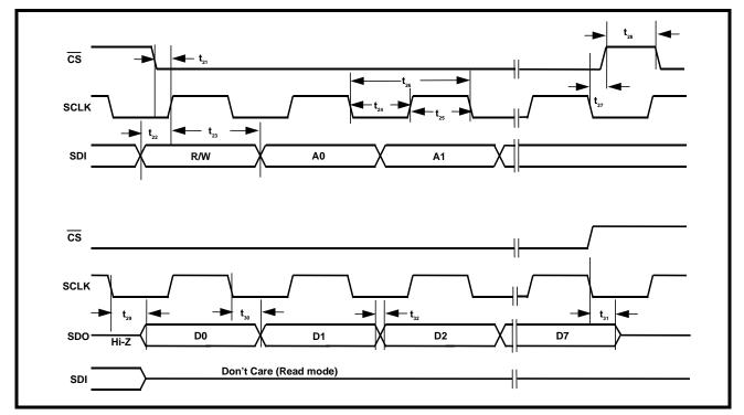
FIGURE 11. TIMING DIAGRAM FOR THE MICROPROCESSOR SERIAL INTERFACE
