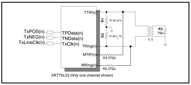
When the MTIP\_n and MRing\_n are connected to the TTIP\_n and TRing\_n lines, the drive monitor circuit monitors the line for transitions. The DMO\_n (Drive Monitor Output) will be asserted "Low" as long as the transitions on the line are detected via MTIP\_n and MRing\_n.
