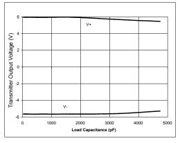
SP3224E/SP3226E Transmitter Output Voltage vs. Load Capacitance
