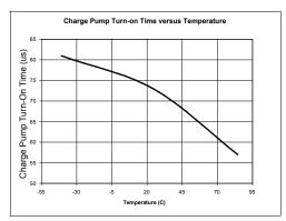
Charge Pump Turn-On Time vs. Temperature
