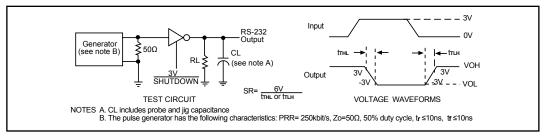
Figure 1. Driver Slew Rate
