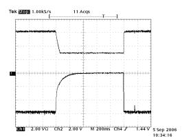
SP3224E/SP3226E Charge Pump Into Shutdown
