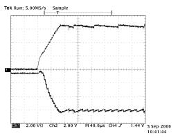
SP3225E/SP3227E Charge Pump Power On Time, Vcc=3.3V
