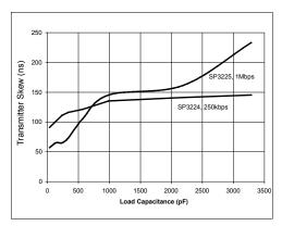
Driver Skew vs. Load Capacitance
