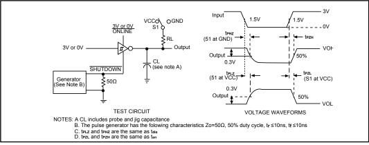
Figure 4. Receiver Enable and Disable Times
