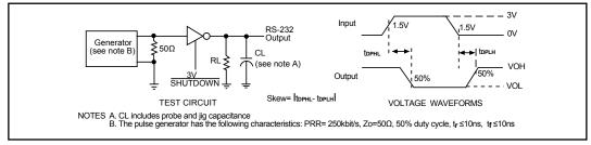
Figure 2. Driver Propagation and Skew
