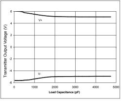
SP3225E/SP3227E Transmitter Output Voltage
