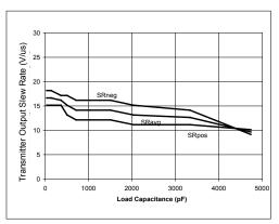
SP3224E/SP3226E Transmitter Output Slew Rate vs. Load Capacitance
