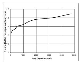
SP3224E/SP3226E Transmitter Input to Receiver Output Propagation Delay vs.
