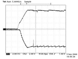
SP3224E/SP3226E Charge Pump Power On Time, Vcc=3.3V
