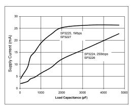
Supply Current vs. Load Capacitance
