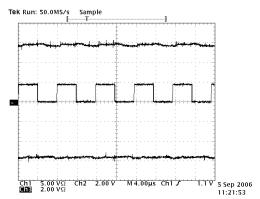
SP3224E/SP3226E Charge Pump Waveforms for 250kbp Clock Rate
