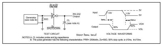
Figure 3. Receiver Propagation Delay and Skew
