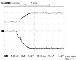
SP3224E/SP3226E Charge Pump Out of Shutdown
