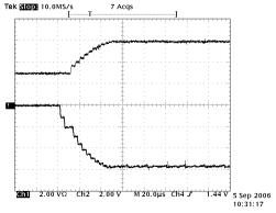
SP3225E/SP3227E Charge Pump Out of Shutdown
