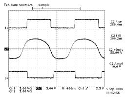
SP3225E/SP3227E Waveforms for 1Mbps Clock Rate, RL=3K $\Omega$ , CL=1000pF
