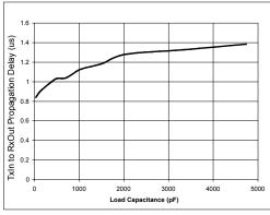
SP3225E/SP3227E Transmitter Input to Receiver Output Propagation Delay vs.
