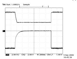
SP3225E/SP3227E Charge Pump Into Shutdown
