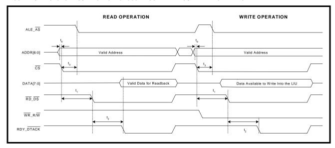
TABLE 52: ASYNCHRONOUS - MOTOROLA 68K - INTERFACE TIMING SPECIFICATION
