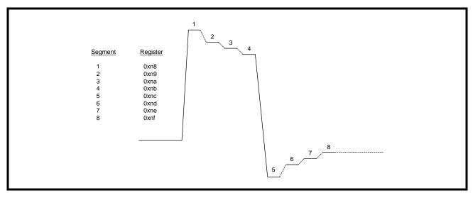
By default, the arbitrary segments are programmed to 0x00h. The transmitter outputs will result in an all zero pattern to the line. For E1 arbitrary mode, see global register 0xC0h.
