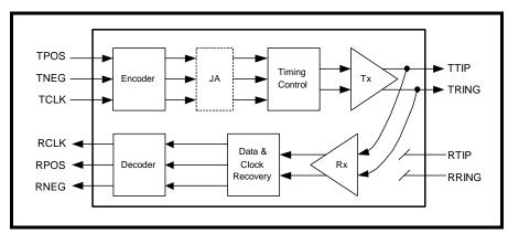
In this mode, the jitter attenuator (if selected) can be placed in the transmit or receive path.
