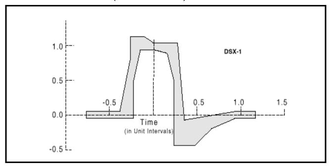
TABLE 49: DSX1 INTERFACE ISOLATED PULSE MASK AND CORNER POINTS
