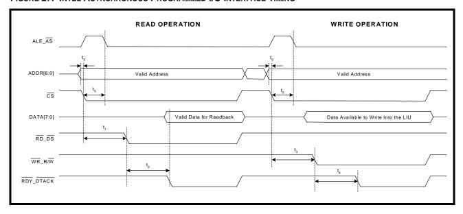
TABLE 51: ASYNCHRONOUS MODE 1 - INTEL 8051 AND 80188 INTERFACE TIMING
