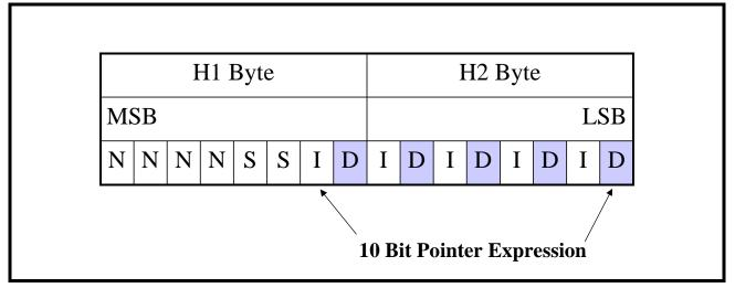
**Note:** At this time the "D" bits are inverted in order to denote that a "decrementing" pointer adjustment event is currently occurring.
