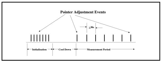
Telcordia GR-253-CORE states that the Intrinsic Jitter that is measured (within the DS3 signal) that is ultimately de-mapped from a SONET signal that is experiencing "Single-Pointer Adjustment" events, must NOT exceed the value 0.3UI-pp + Ao.
