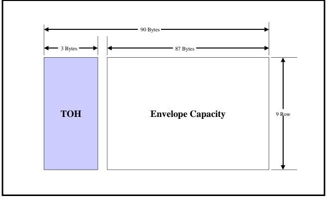
Since the TOH bytes occupy the first three byte columns of each STS-1 frame, and since each STS-1 frame consists of nine (9) rows, then we can state that the TOH (within each STS-1 frame) consists of 3 byte columns x 9 rows = 27 bytes. The byte format of the TOH is presented below in Figure 33.
