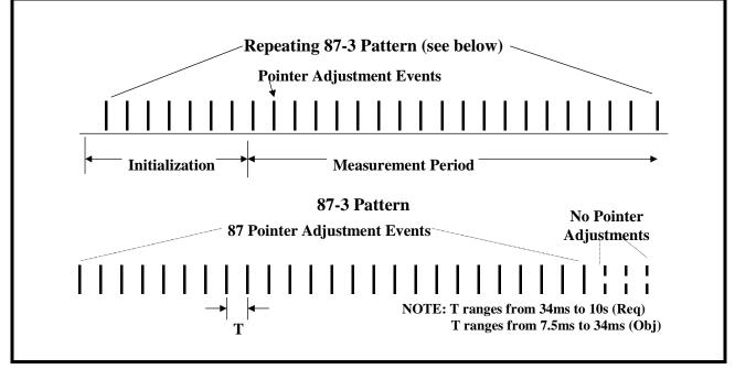
Telcordia GR-253-CORE defines an "87-3 Continuous" Pointer Adjustment pattern, as a repeating sequence of 90 pointer adjustment events. Within this 90 pointer adjustment event, 87 pointer adjustments are actually executed. The remaining 3 pointer adjustments are never executed. The spacing between individual pointer adjustment events (within this scenario) can range from 7.5ms to 10seconds.
