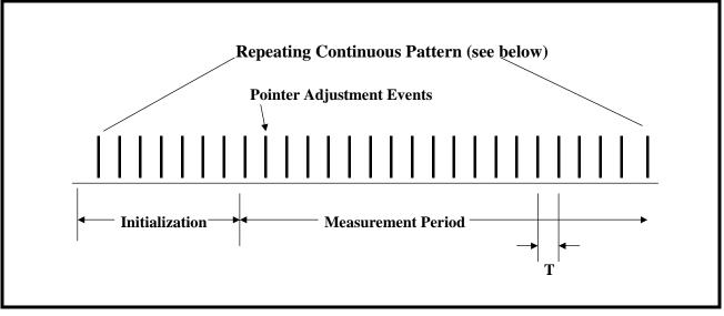
Telcordia GR-253-CORE mandates that the Intrinsic Jitter, within the DS3 signal that is de-mapped from a SONET signal, which is experiencing the "Continuous" pattern of Pointer Adjustments, must not exceed 1.0UIpp. The spacing between individual pointer adjustments (within this scenario) can range from 7.5ms to 10s.
