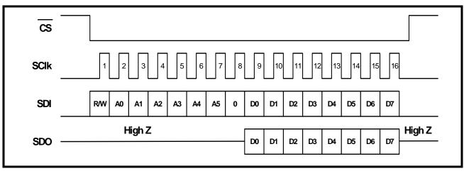
FIGURE 11. TIMING DIAGRAM FOR THE MICROPROCESSOR SERIAL INTERFACE
