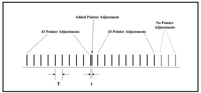
Telcordia GR-253-CORE defines an "87-3 Add" Pointer Adjustment, as the "87-3 Continuous" Pointer Adjustment pattern, with an additional pointer adjustment inserted, as shown above in Figure 52.
