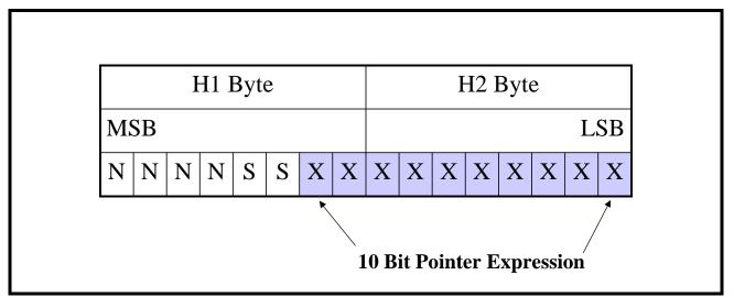
Figure 43 relates the contents within these 10 bits (within the H1 and H2 bytes) to the location of the J1 byte (e.g., the very first byte of the STS-1 SPE) within the Envelope Capacity.
