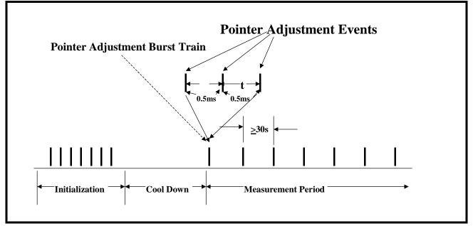
Telcordia GR-253-CORE mandates that the Intrinsic Jitter, within the DS3 signal that is de-mapped from a SONET signal, which is experiencing the "Burst of Pointer Adjustment" scenario, must NOT exceed 1.3UI-pp.
