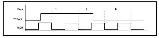
In Dual-Rail mode, data is input via TPData and TNData pins. TPData contains positive data and TNData contains negative data. The SR/DR input pin = "Low" (in Hardware Mode) or bit 0 of the control register = "0" (in Host Mode) enables the Dual-Rail mode. Figure 13 illustrates the Dual-Rail data format.
