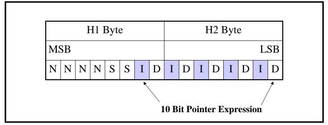
**Note:** At this time the "I" bits are inverted in order to denote that an "incrementing" pointer adjustment event is currently occurring.
