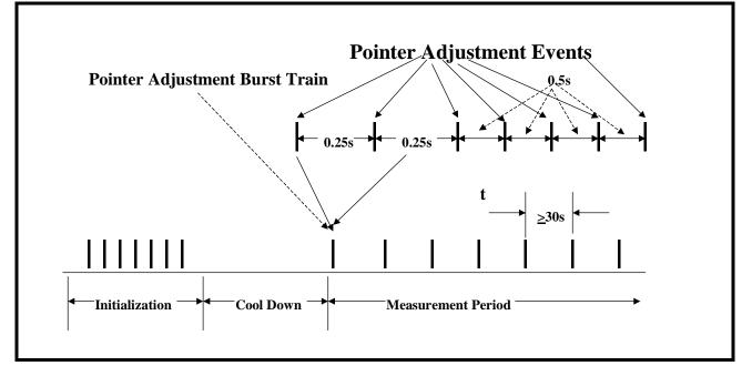
Telcordia GR-253-CORE mandates that the Intrinsic Jitter, within the DS3 signal that is de-mapped from a SONET signal, which is experiencing the "Phase Transient - Pointer Adjustment" scenario must NOT exceed 1.2UI-pp.
