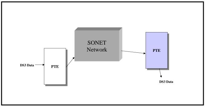
As mentioned above a DS3 or E3 signal will be asynchronously mapped into a SONET or SDH signal and then transported over the SONET or SDH network. At the remote PTE this DS3 or E3 signal will be extracted (or de-mapped) from this SONET or SDH signal, where it will then be routed to DS3 or E3 terminal equipment for further processing.
