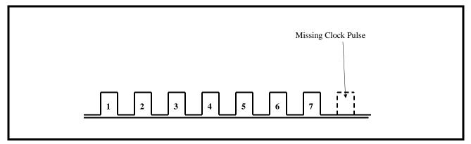
It should be noted that each of these clock pulses has a period of approximately 19.3ns (or has an "instantaneously frequency of 51.84MHz).
