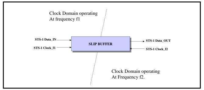
In the "Slip Buffer, the "input" STS-1 data (labeled "STS-1 Data\_IN") is latched into the FIFO, upon a given edge of the corresponding "STS-1 Clock\_f1" input clock signal. The STS-1 Data (labeled "STS-1 Data\_OUT") is clocked out of the Slip Buffer upon a given edge of the "STS-1 Clock\_f2" input clock signal.
